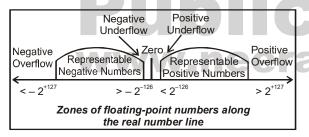
Numbers greater than  $2^{+127}$  cannot be represented; this is called *positive overflow*. A similar range of negative numbers can be represented. Numbers to the left of that range cannot be represented; this is negative overflow. There is also a range of numbers near zero that cannot be represented.
