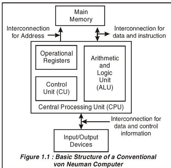
Figure 1.1 : Basic Structure of a Conventional von Neuman Computer
